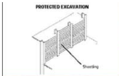
Deeper excavations require engineered protective systems
