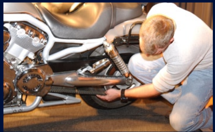
Keep the chain at the proper tension and alignment (refer to your owner's manual) and lubricate it often. Photo courtesy of the Motorcycle Safety Foundation.
