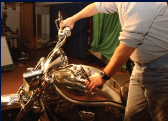
Controls should be smooth and cables should not be kinked or frayed.
