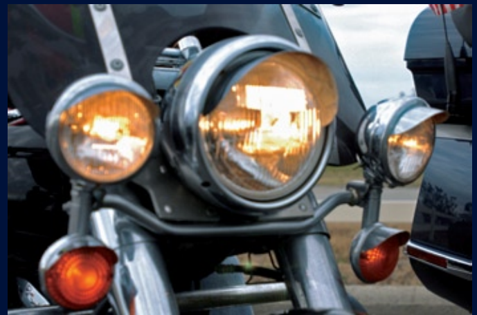
Your headlight should work properly and be aimed correctly on both-high and low-beam settings.
