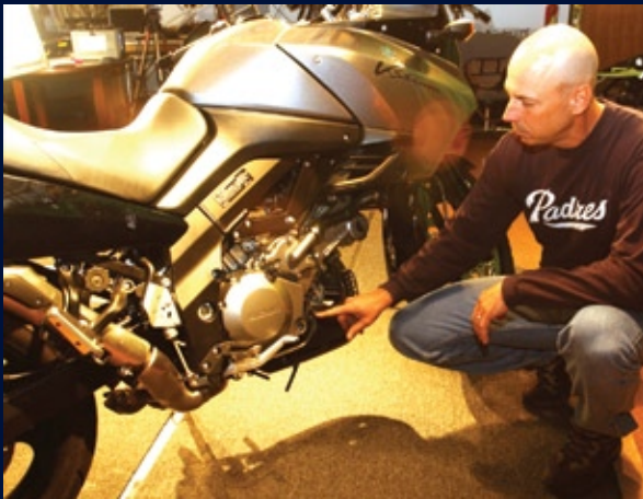
The oil in most street bikes lubricates the engine as well as the transmission, so it's doubly important to make sure the oil level is correct.
