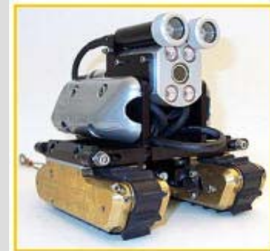
Example of a robot inspection unit ( courtesy of Inuktun ServicesLtd )
