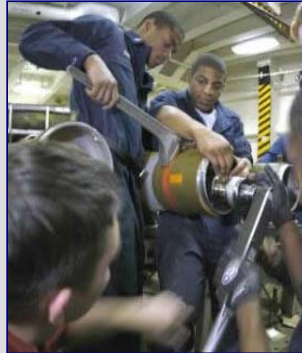
Sailors assigned to the Weapons Department attach a laser guidance unit to a BLU-111 500-pound general-purpose bomb in an ammunition magazine aboard USS Kitty Hawk (CV 63).
