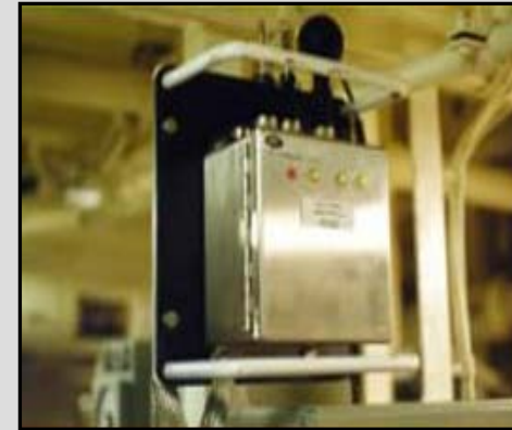
The Automated Heat Stress System (AHSS) measures dry bulb temperature, globe temperature and relative humidity, calculates the WBGT and displays PHEL stay times.
