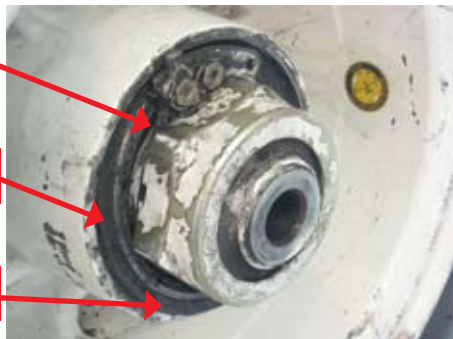
Missing metal spacer
