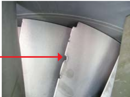
Damaged engine blades
