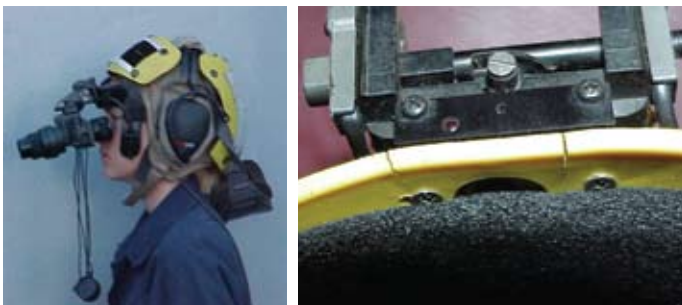
Left: One of several fleet "fixes" to NVD mounting (note poor eye alignment, snag hazards). Right: Crack in cranial impact shield from NVD mount.
