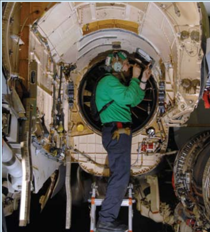
AE3 Stephen Bell, assigned to the “Kestrels” of VFA-137, performs maintenance on the engine bay of an FA-18E Super Hornet aboard the Nimitz -class aircraft carrier USS Abraham Lincoln (CVN-72). Navy photo by MC3 Rialyn Rodrigo
