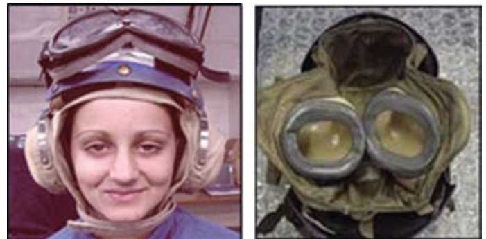
Largest cranial does not fit all (cranial is hard to clean and standard earcup seals harden, crease, and leak noise).
