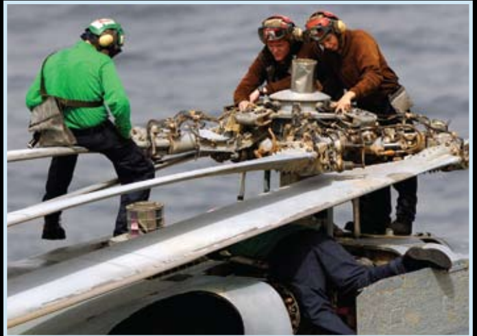
Sailors perform routine maintenance on an SH-60B helicopter assigned to the Saberhawks of HSL-47 on the flight deck of the Nimitz -class aircraft carrier USS Abraham Lincoln (CVN-72). Navy photo by MC3 Geoffrey Lewis
