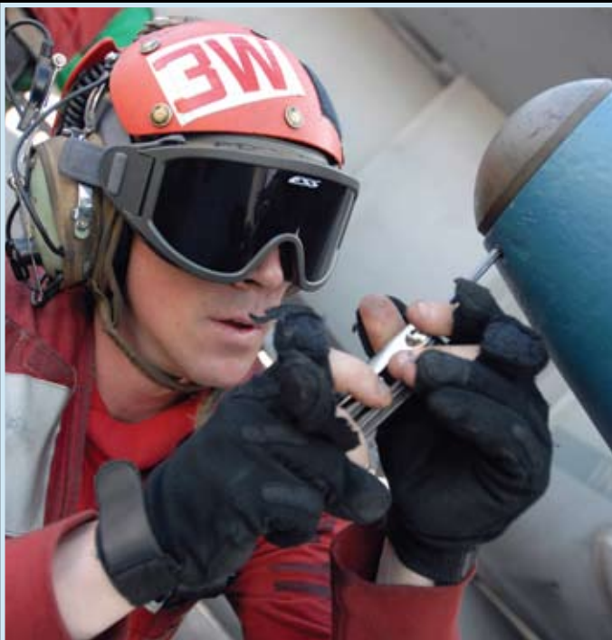
AO2 David Mathews installs a set screw after replacing a nose plug on a laser-guided bomb unit (GBU) 32 aboard the Nimitz -class nuclear-powered aircraft carrier USS Ronald Reagan (CVN-76). Navy photo by MC3 Gary Prill
