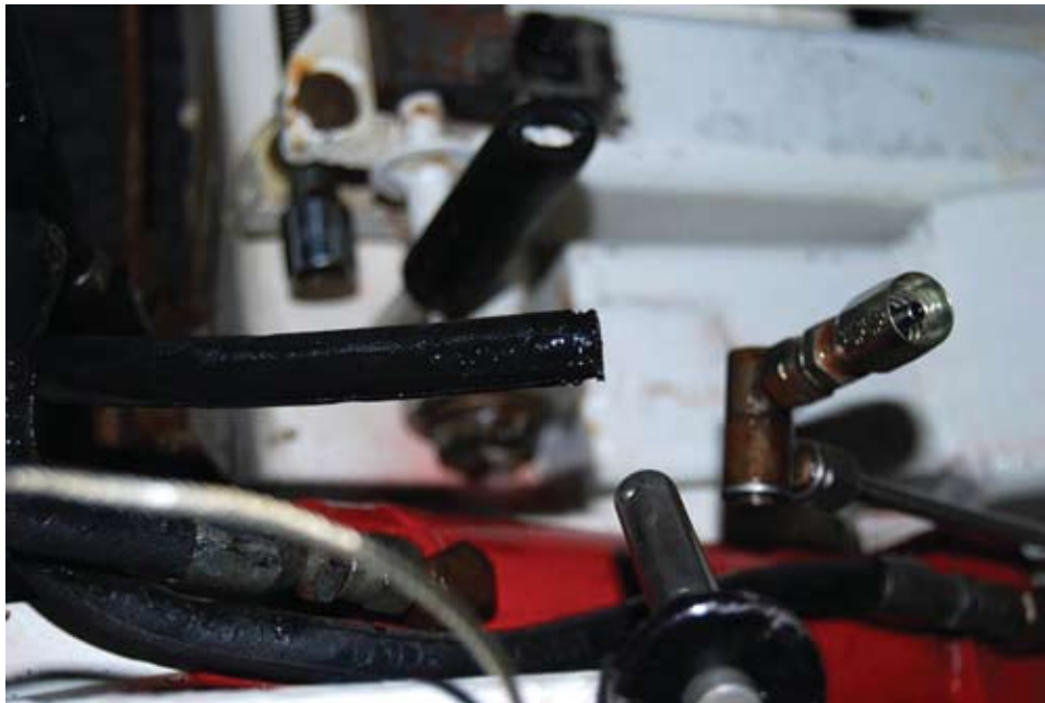
Aft hydraulic line on ETU-110 failure (above).
