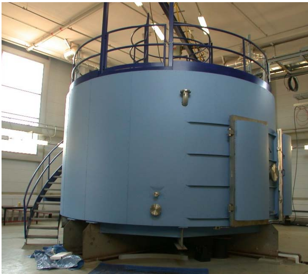
Fig. 5.3-6. Evacuated scattering chamber.
