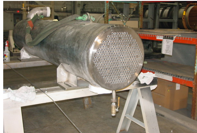
Fig. 5.2-18. Double-wall mercury-water heat exchanger schematic and fabrication prior to welding end caps.
