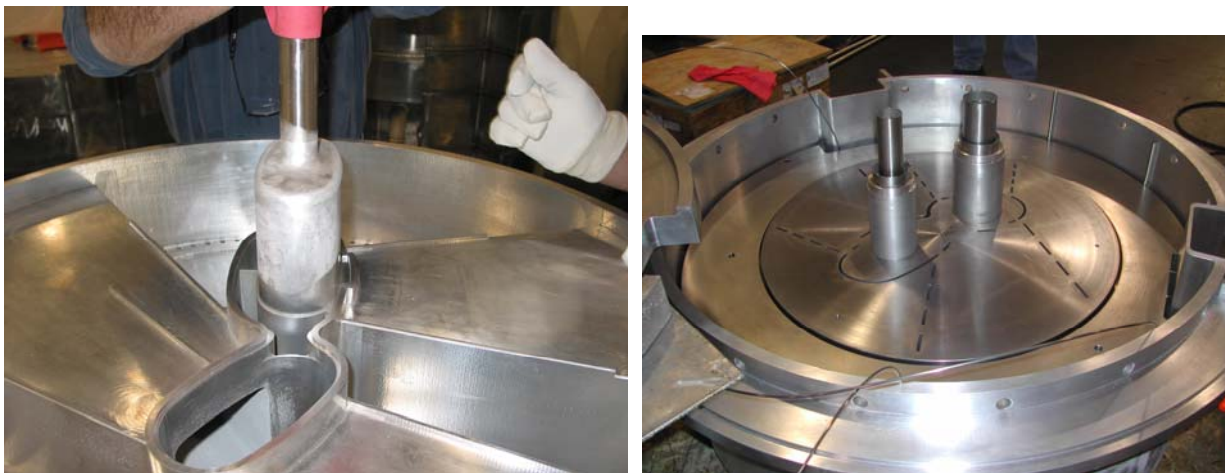
Fig. 5.2-35. Moderators being installed in the inner reflector plug.
