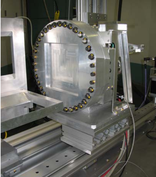
Fig. 5.3-18. Scattered beam: (a) ^3\text{He} area detector, (b) ^3\text{He} polarization analyzer and neutron detector installed on goniometer system.
