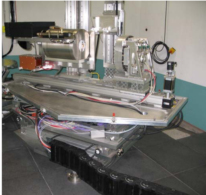
Fig. 5.3-18. Scattered beam: (a) ^3\text{He} area detector, (b) ^3\text{He} polarization analyzer and neutron detector installed on goniometer system.
