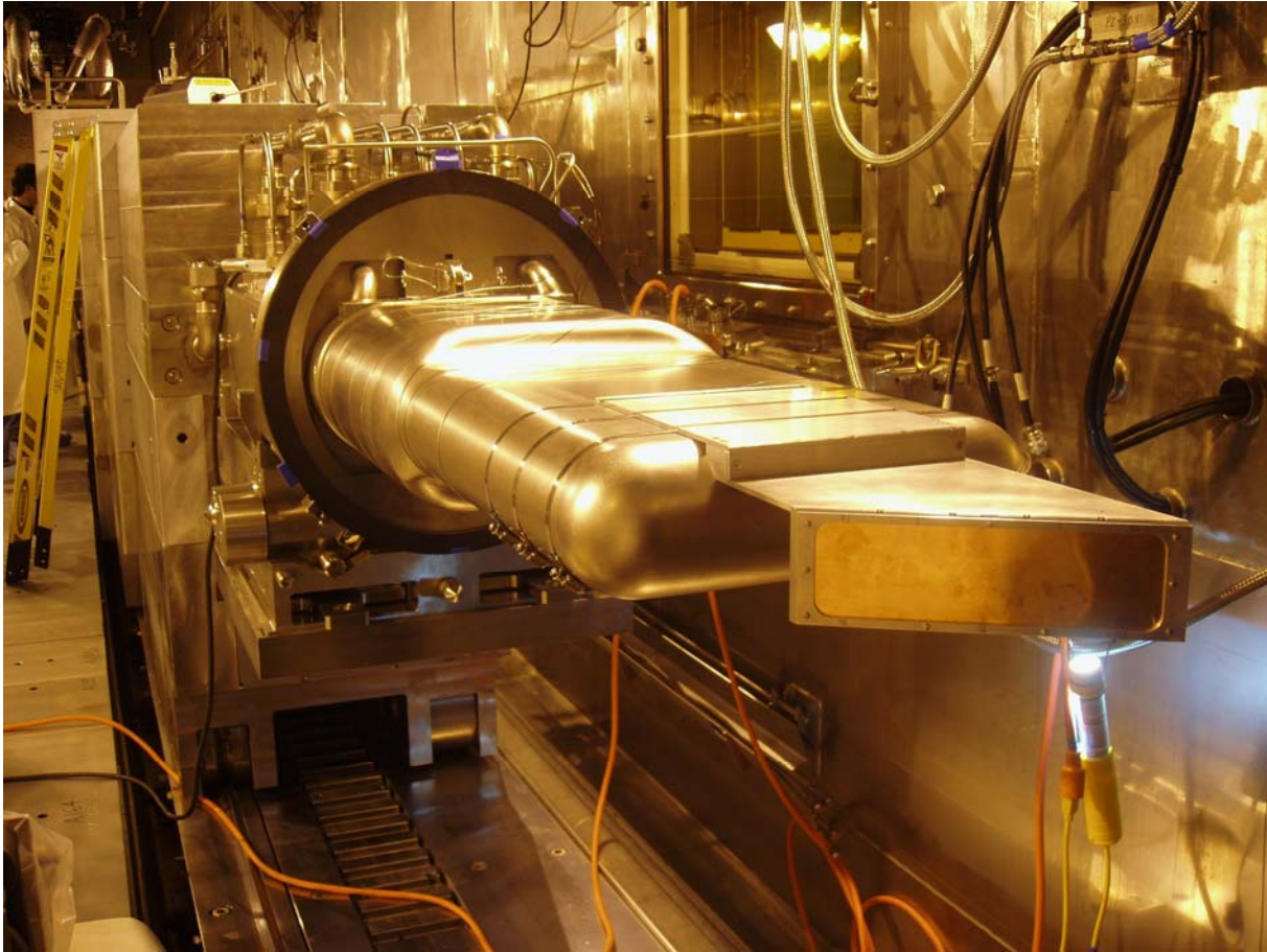
Fig. 5.2-24. Phosphor viewscreen installed on front of target module.
