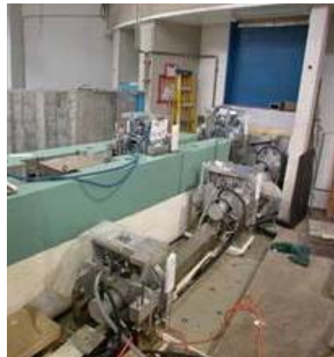
Fig. 5.3-19. Incident beam: (a) neutron guide system installed on downward-inclined beam line; (b) three choppers installed in spaces in guide system.
