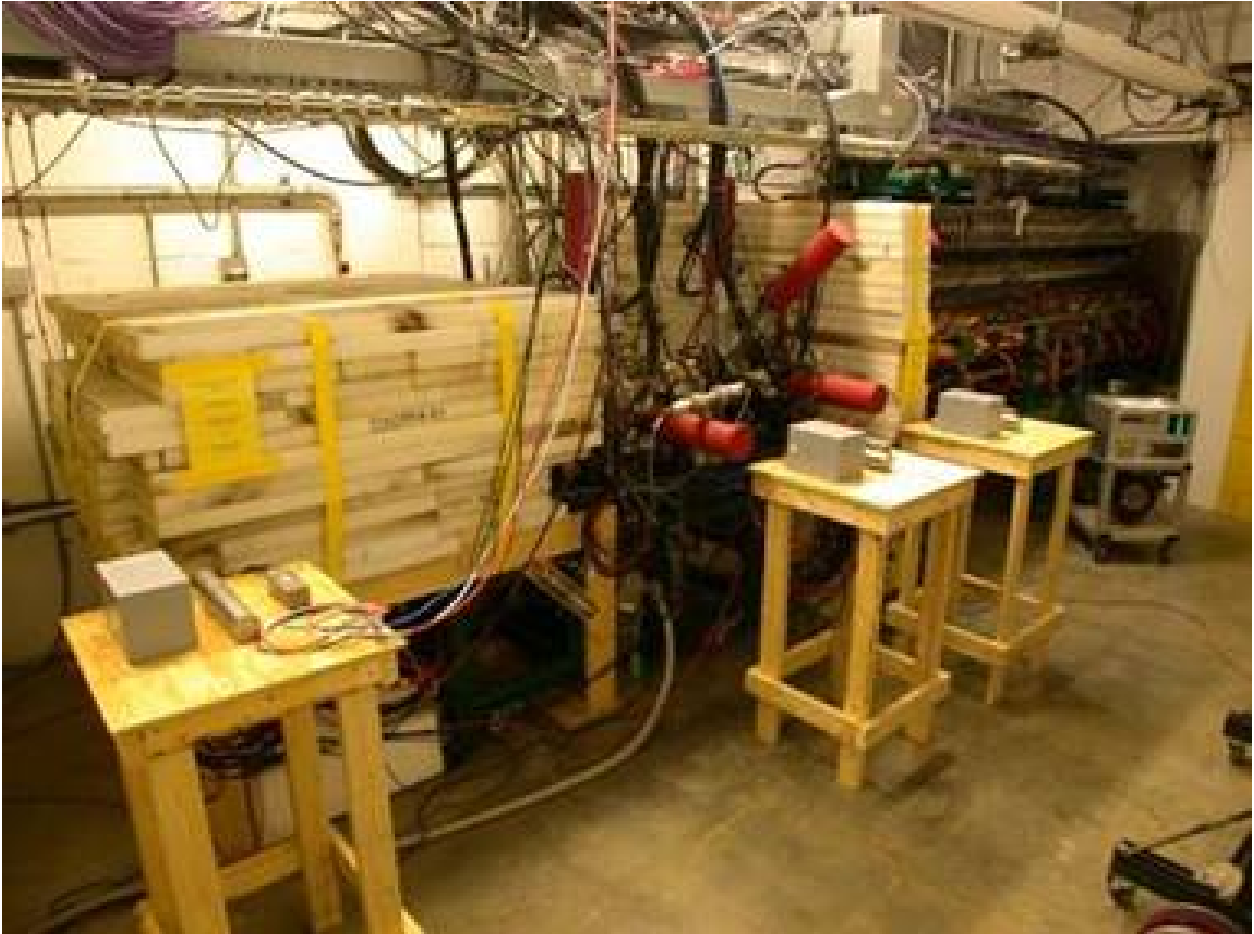
Fig. 5.1-5. Attached to the FES is the first DTL tank with a diagnostics section and a 12-kW beam dump attached. This was used to fully characterize the beam.
