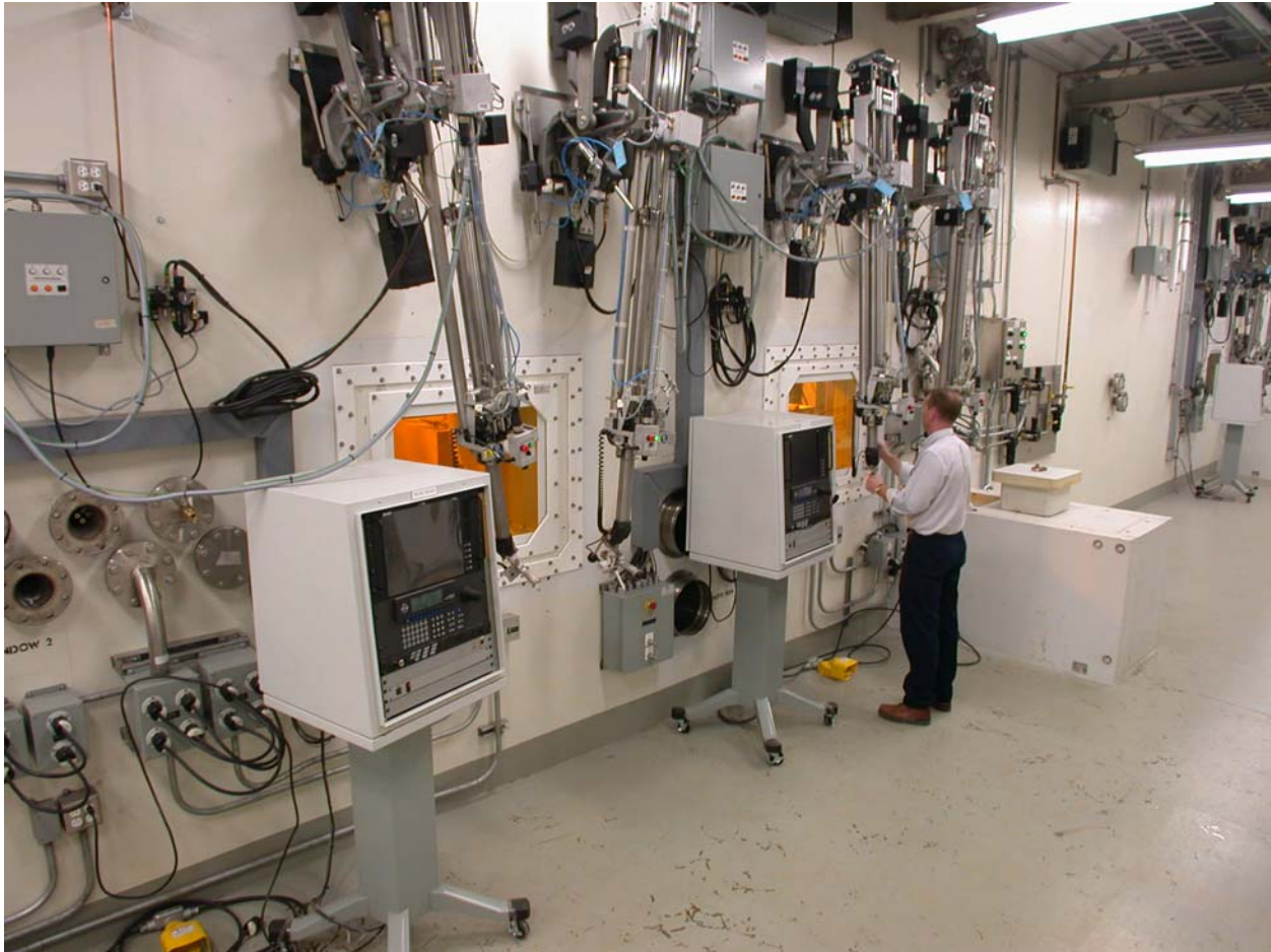
Fig. 5.2-62. Workstations 2 and 3 showing windows, CRL manipulators, and video monitors.
