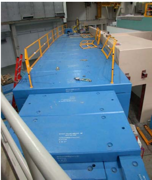
Fig. 5.3-5. Beam line shielding: (a) heavily shielded initial curved guide section; (b) lighter shielding beyond the fast neutron line of sight.
