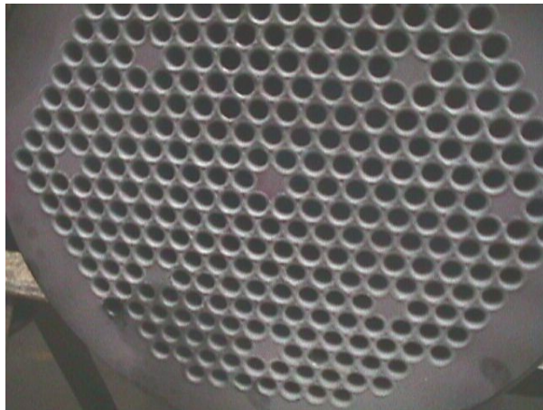
Fig. 5.2-18. Double-wall mercury-water heat exchanger schematic and fabrication prior to welding end caps.
