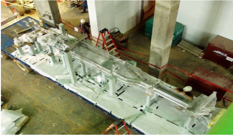
Delivery of the mercury and utility piping assembly. The fixture is designed to allow manufacture of replacement piping.
