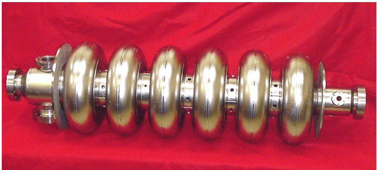
Fig. 5.1-17. Niobium cavity for the superconducting accelerator.
