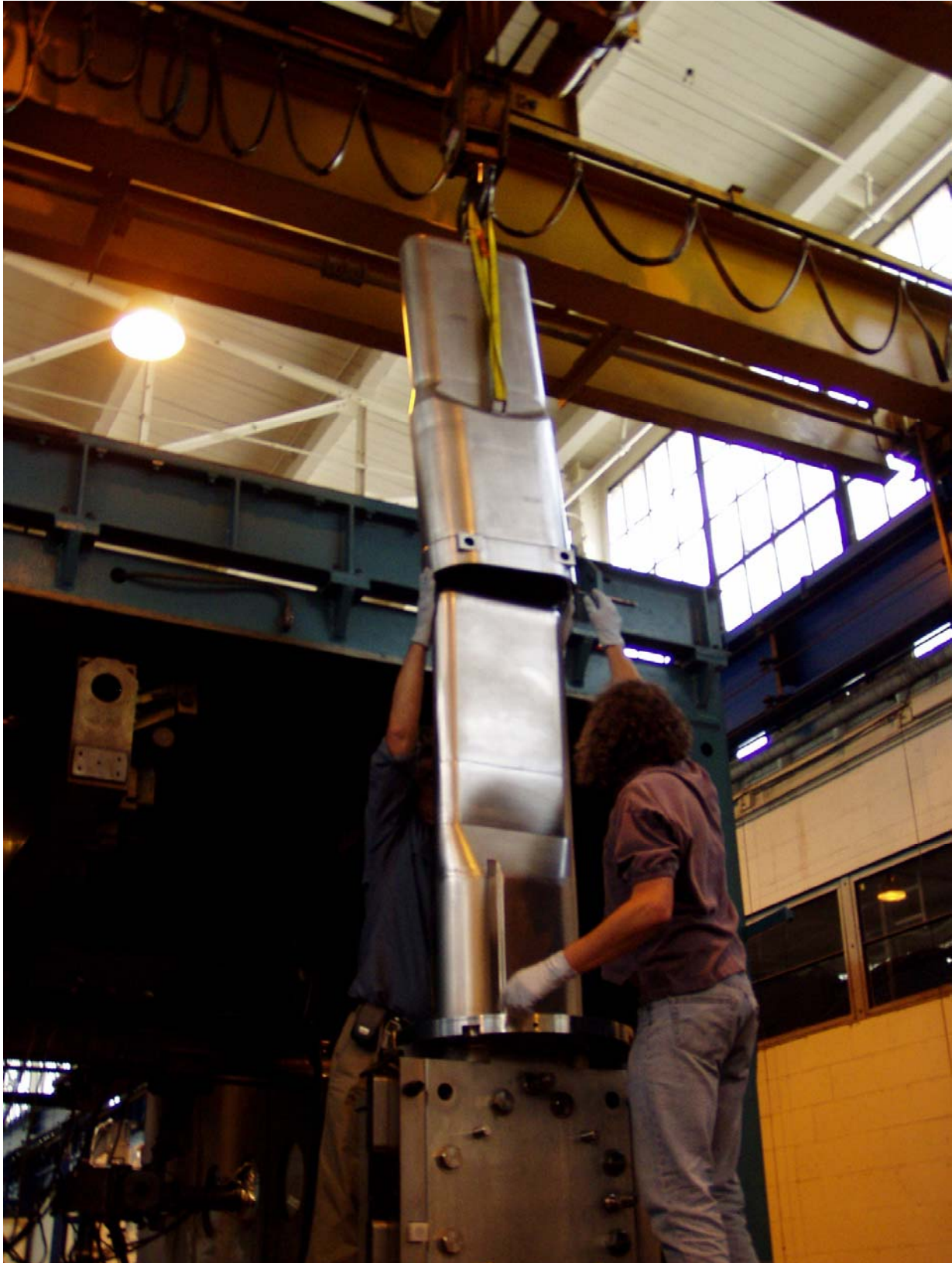
Fig. 5.2-5 .Target module mercury vessel and water shroud before welding.
