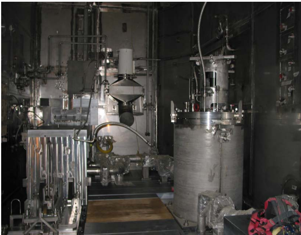
Fig. 5.2-20. Target carriage in operating position and mercury pump.
