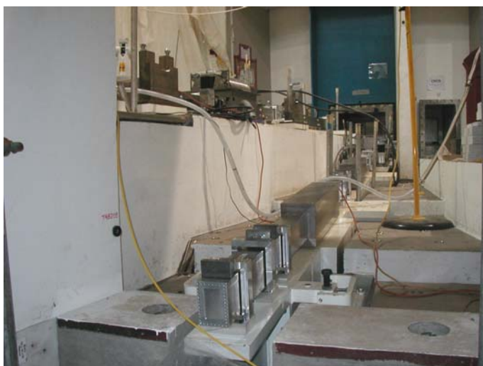
Fig. 5.3-19. Incident beam: (a) neutron guide system installed on downward-inclined beam line; (b) three choppers installed in spaces in guide system.
