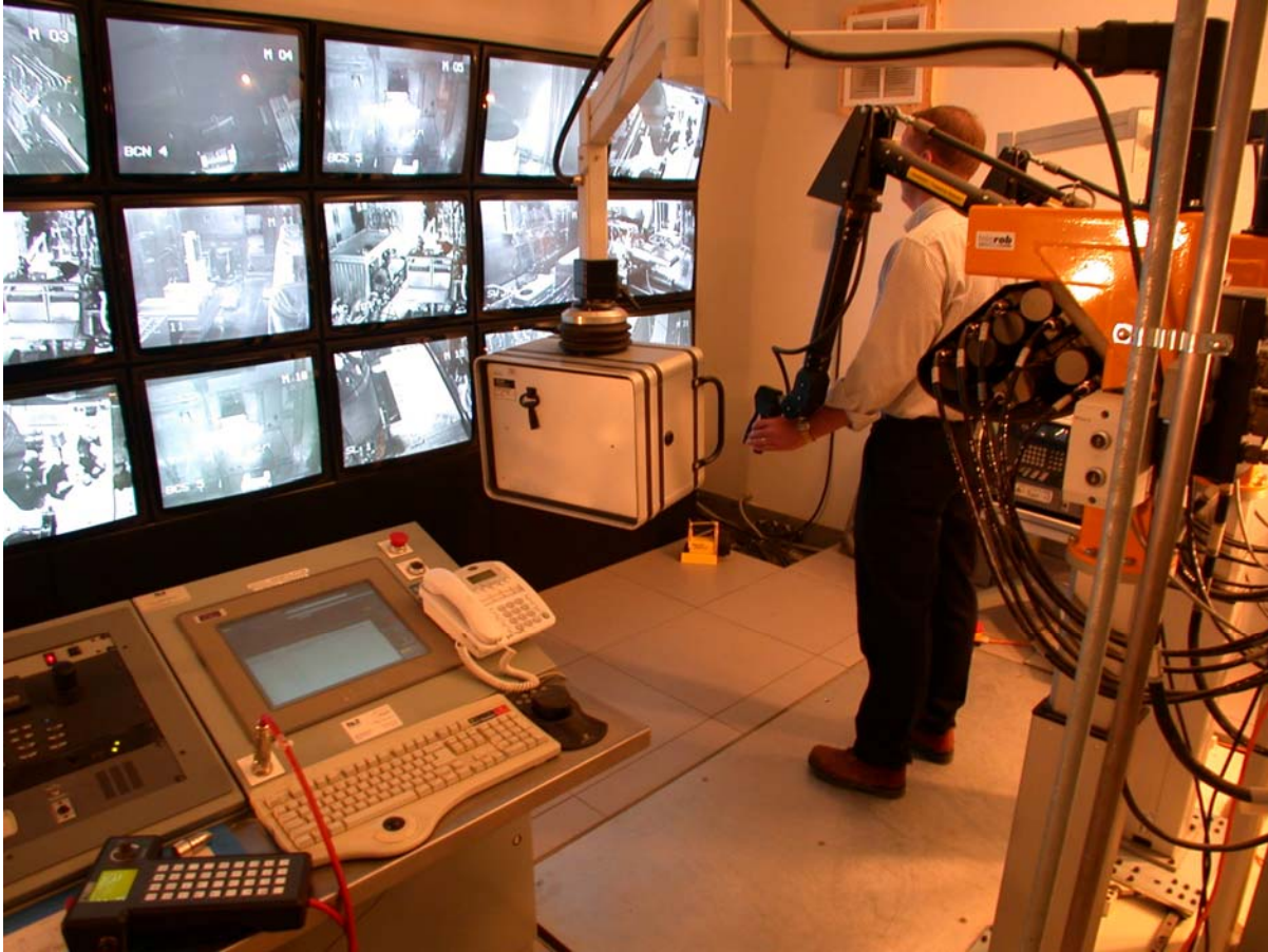
Fig. 5.2-65. Servomanipulator station in remote-handling control room.
