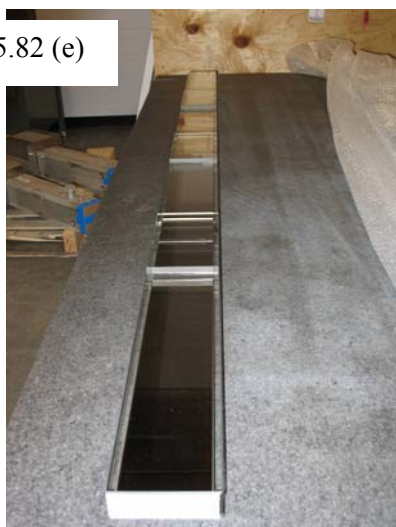
Fig. 5.3-24. Components for the Powder Diffractometer: (a) secondary shutter; (b) insert for secondary shutter; (c) poured-in-place shielding; (d) bulk shield insert; (e) section of guide; (f) first detector module.
