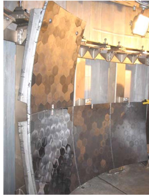
Fig. 5.3-7. Silicon crystal arrays: (a) gluing crystals to one panel; (b) four panels mounted in instrument.
