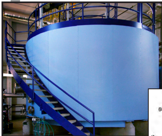
Backscattering spectrometer large evacuated final flight path.
