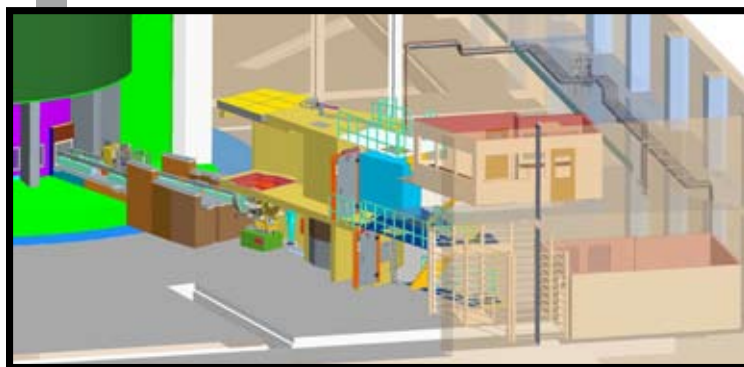
Engineering model of VISION, including T_0 chopper, bandwidth chopper, secondary spectrometer, and utility rooms.
