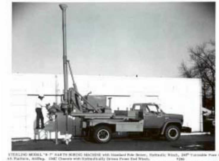
Figure #1. This is not the truck-mounted auger that was used in this operation, but it is an example of this type of equipment. Notice the operator platform at the rear.
