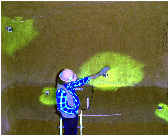
A Los Alamos scientist examines the migration of dye-laced water injected into unsaturated rock. These studies confirmed the conceptual model for water movement through the unsaturated tuffs of Yucca Mountain.
