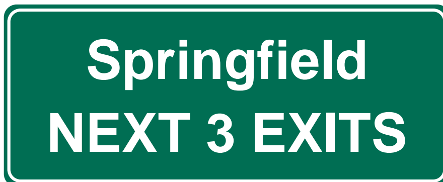
Figure 2E-24. NEXT EXITS Sign
