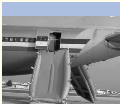
Aircraft evacuation slides have been upgraded to better resist heat from post-crash fires.
