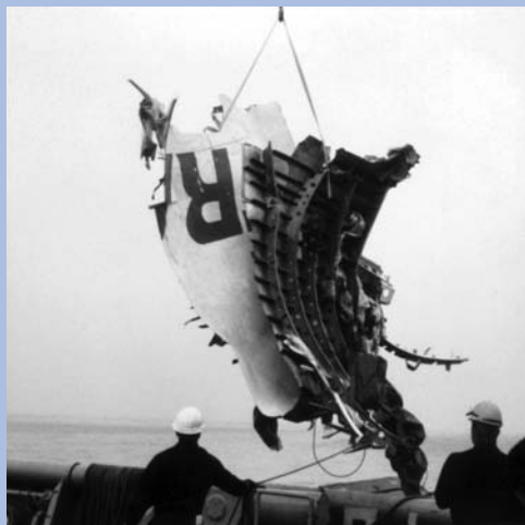
A fuel-air vapor explosion in the center wing tank of a 747 brought down the plane in 1996, killing all 230 on board.
