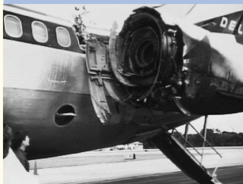
Debris from an engine that failed during takeoff punctured the cabin of a MD-88 in 1996, killing two passengers. Improvements in engine inspection and training resulted from the accident.
