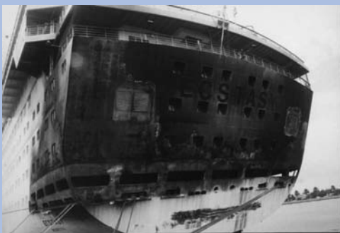
NTSB investigators probed the 1998 fire aboard a cruise ship that heavily damaged the ship shortly after it left the Port of Miami.
