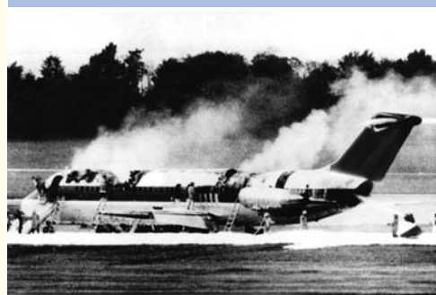
Fire aboard a DC-9 in 1983 led to smoke detectors in lavatories and floor-level escape lighting.
