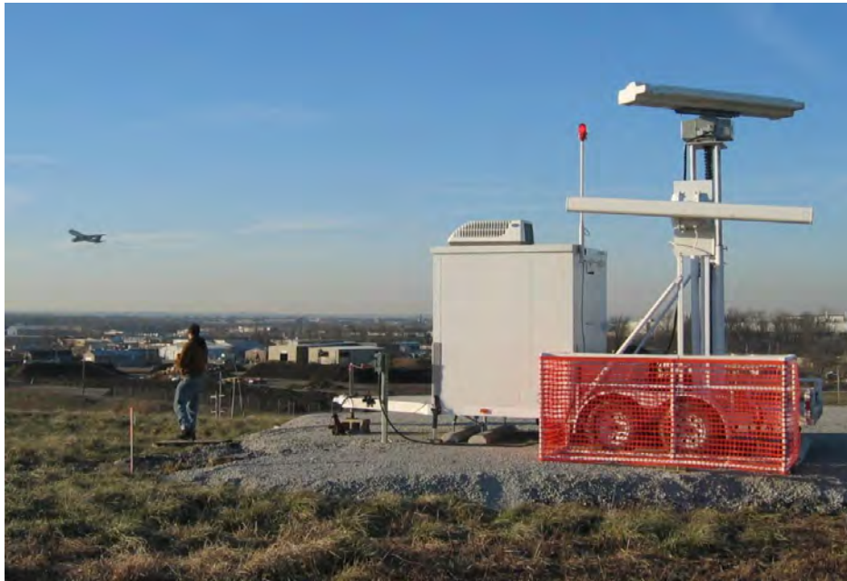
Figure 8. Small Mobile Avian Radar deployed on a landfill, monitoring bird activity on and around the property. This unit uses both vertical and horizontal scanning radars to collect area and height data simultaneously.
