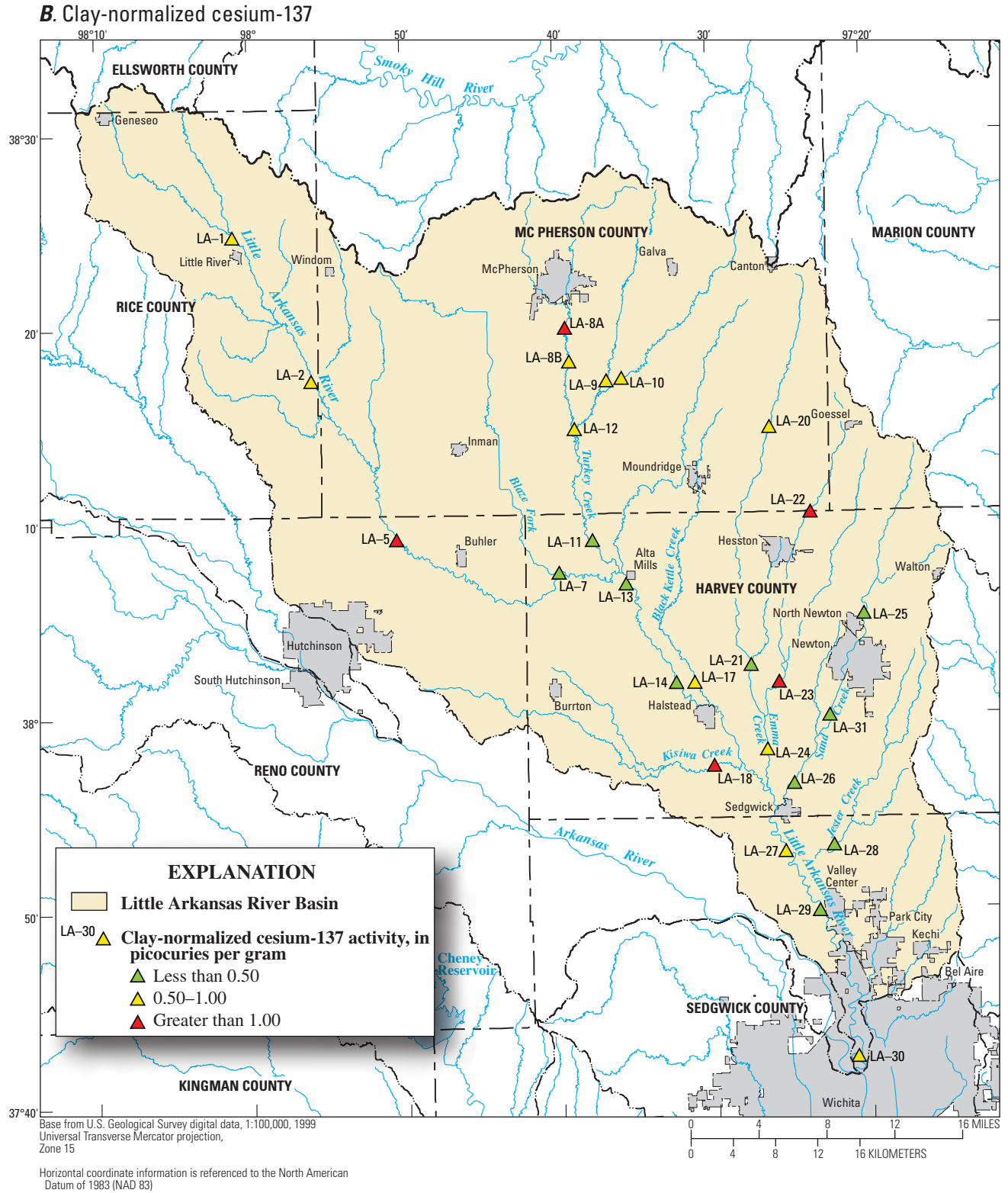
Figure 10. Original (A) and clay-normalized (B) cesium-137 activity in streambed-sediment samples collected in the Little Arkansas River Basin, south-central Kansas, January and March 2007.—Continued
