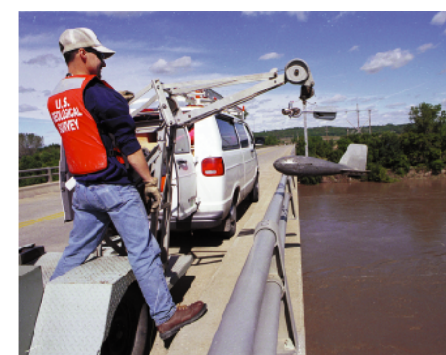
Discharge measurements made during floods are used to develop stage-discharge relations at each gaging station. (Photograph, Lawrence Journal World, Lawrence, Kans.)
