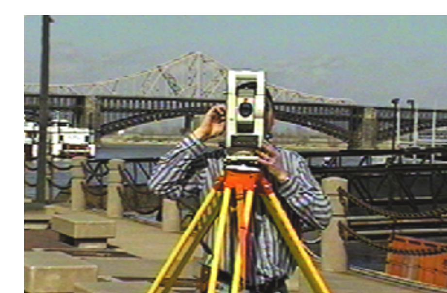
Some floods are measured by USGS hydrographers using indirect methods that involve surveys of valley cross sections, bridge-opening measurements, and high-water marks that are used in mathematical flow equations to compute discharge.
