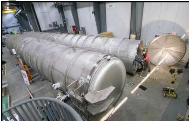
Detector tanks for the new SANS instruments at HFIR. The Bio-SANS detector is on the left.
