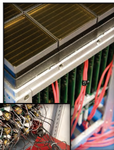
Top right: View inside an Anger camera showing the input windows of the position-sensitive photomultiplier tubes and their preamplifier boards.
