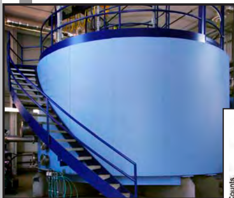
Backscattering spectrometer large evacuated final flight path.
