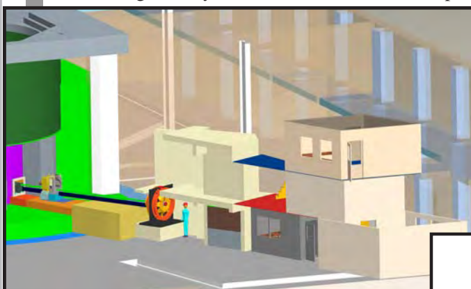
Engineering model of VISION, including T_0 chopper, bandwidth chopper, secondary spectrometer, and utility rooms.
