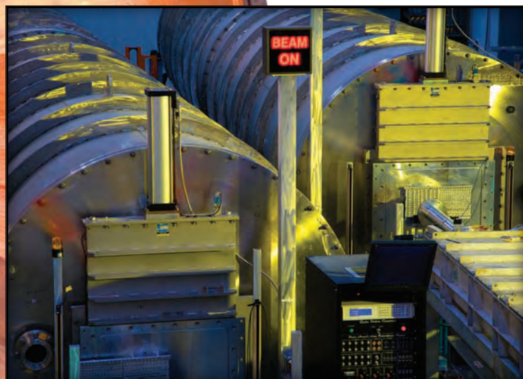
Detector tanks for the new SANS instruments at HFIR. On the left is the tank for the general-purpose, high-resolution instrument; the tank on the right is for the Bio-SANS instrument, which is constructed specifically for biological research.
