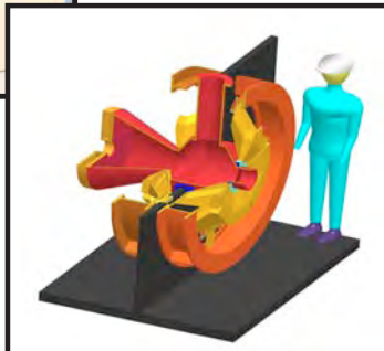
Secondary spectrometer with detector and analyzer modules.
