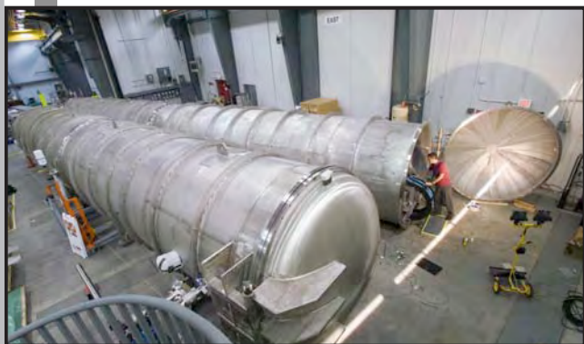
Detector tanks for the new SANS instruments at HFIR. The Bio-SANS detector is on the right.
