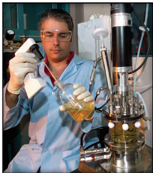
CSMB postdoc Kevin Weiss uses a laboratory scale fermentor to culture organisms in isotopically labeled growth media to produce biomolecules for neutron scattering studies.
