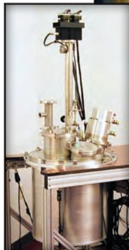
Cryogenic sample changer (FERNS) for the SNS Powder Diffractometer (POWGEN).
