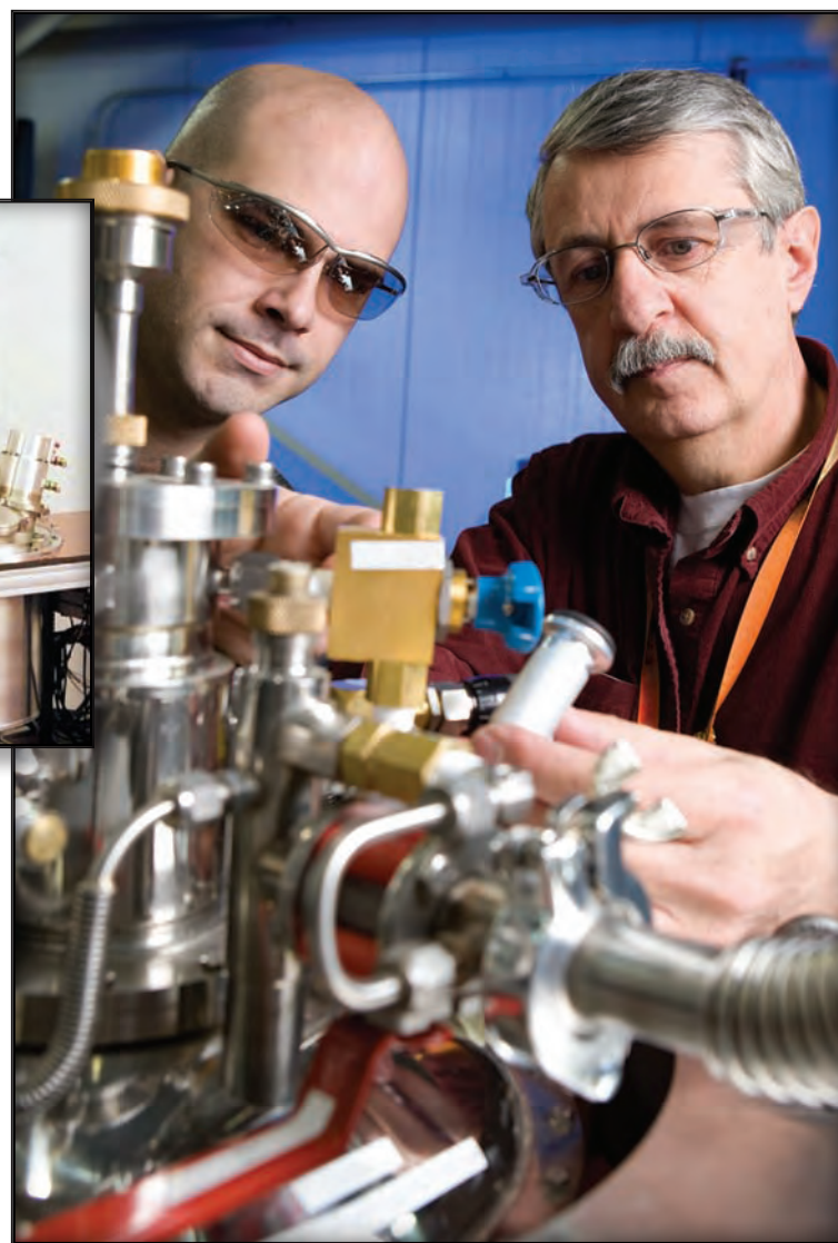
Landon Solomon (left) and Bruce Hill (right) prepare a liquid helium cryostat that will be used to hold a research sample in the neutron beam.
