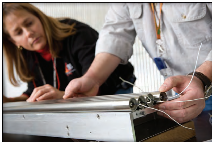
Pam Morrison and Will Reynolds of the SNS Detectors Group install a 2-meter-long LPSD into 8-packs for the Cold Neutron Chopper Spectrometer on beam line 5.
