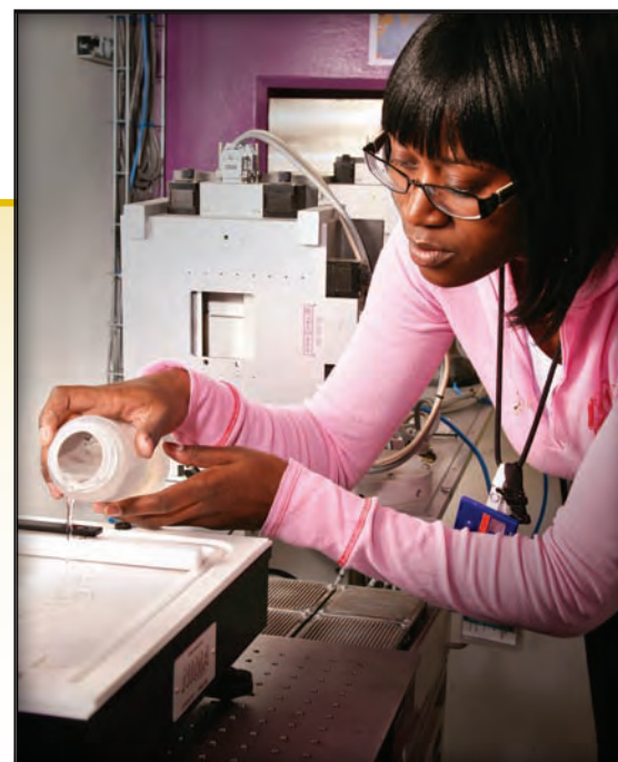
Candice Halbert, scientific associate for the Liquids Reflectometer, fills a Langmuir trough with water. The trough is essentially a Teflon pool used to form a flat surface for water. Neutrons are reflected from molecules spread on the surface.
