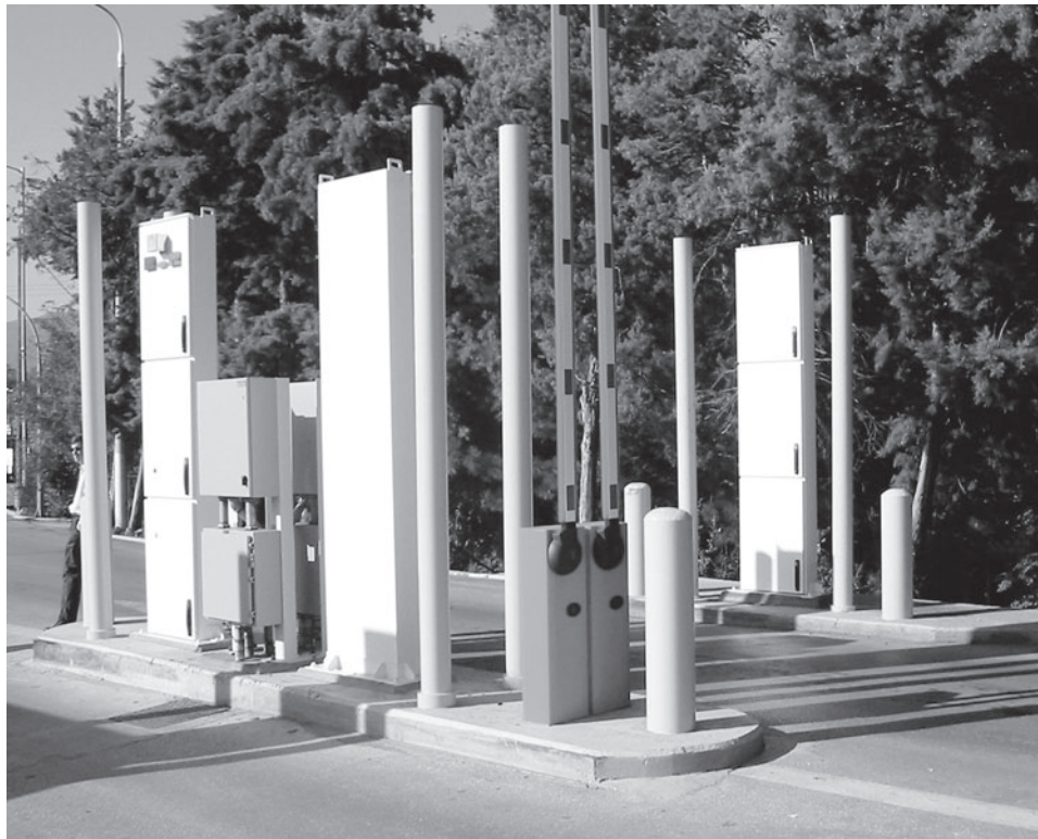
Figure 1: Radiation Portal Monitors Containing Both Gamma and Neutron Radiation Detectors at a Border Site in Northern Greece
