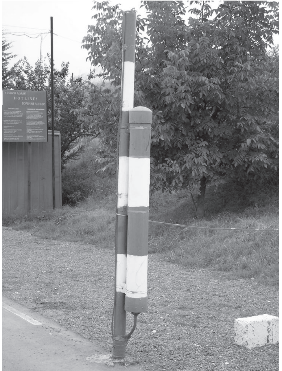
Figure 2: Older Radiation Portal Monitor Able to Detect Only Gamma Radiation at a Border Site in Georgia
