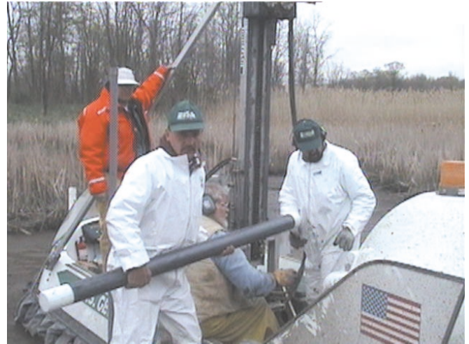
(B) Removing the core in sealed tubes
