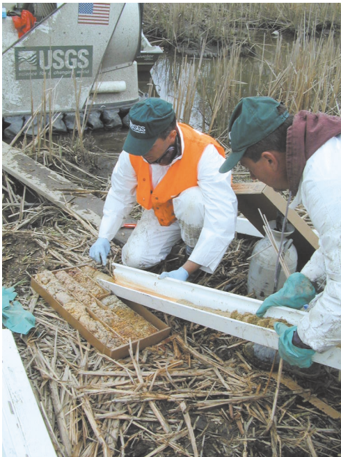
(C) Transferring the core into core boxes
