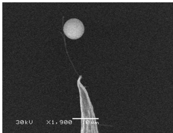
Figure 1. A micrograph of a sphere-nanotube phantom created by NIST. The polystyrene sphere has a diameter of approximately 8 \mu\text{m} and is attached to a tungsten probe tip by a 100 nm double-wall carbon nanotube. This structure was used to compare measured scattering data with analytic results from Mie theory.
