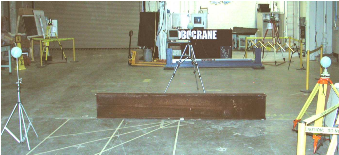
Figure 1: This figure shows the experimental configuration used for scanning an I-beam by a LADAR placed approximately at the camera location. The white lines on the floor are alignment marks for setting the I-beam at different angles relative to the LADAR. The spheres on tripods are located for coordinate registration with a world coordinate system.
