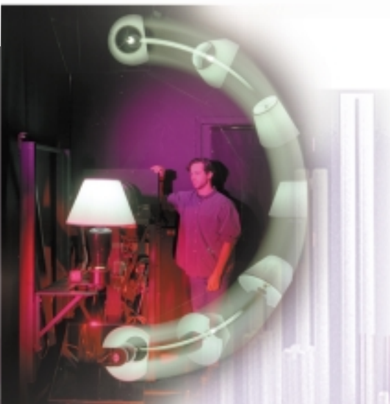
Data from this goniophotometer, developed by EETD researchers to measure the amount of light leaving a fixture at different angles, aid in developing more efficient lighting systems.
