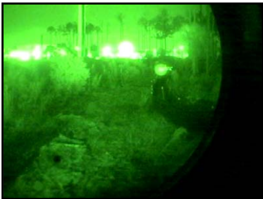
Figure 13. NOD Washout from External Light sources
