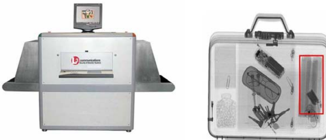
Figure 15. The left image is of a commercially available dual-energy system and the right image is of a briefcase that has alarmed; the area of concern is marked with a red box.
