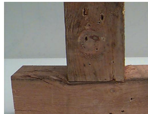
Crush pattern of wood shore
