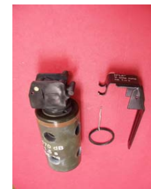
Functioned devices showing ports
