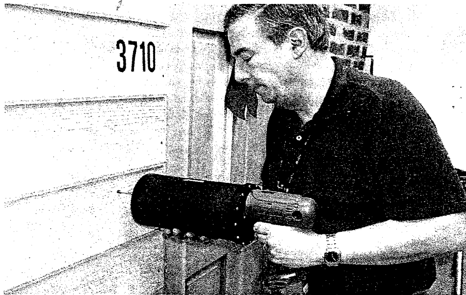
Figure 8. Testing of assembled RADAR Flashlight at GTRI's laboratory test facility
