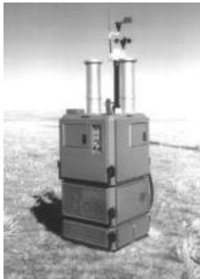
Figure 5-4. Canadian Integrated Biological-Chemical Agent Detection System (CIBADS)/4WARN
