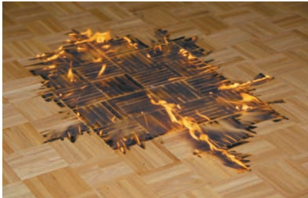
Figure 6. Burning in the cracks of the parquet flooring
