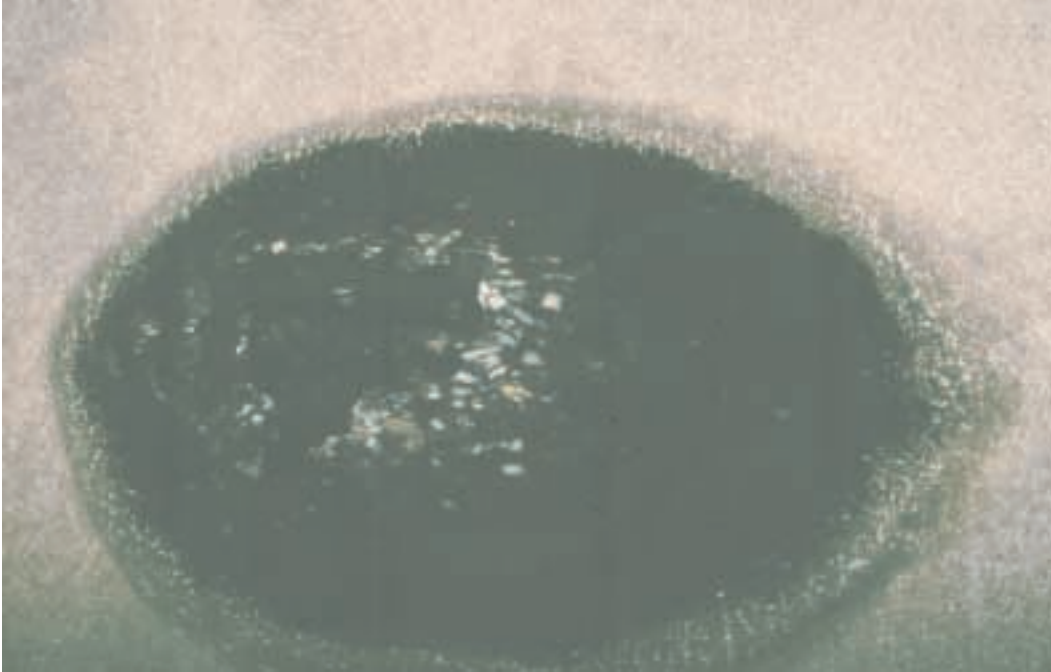
Figure 23. Doughnut burn pattern on carpet 2. 250 mL gasoline fire extinguished at approximately 171 s with CO 2 . Exposed padding can be seen in the center and toward the left side of the pattern.
