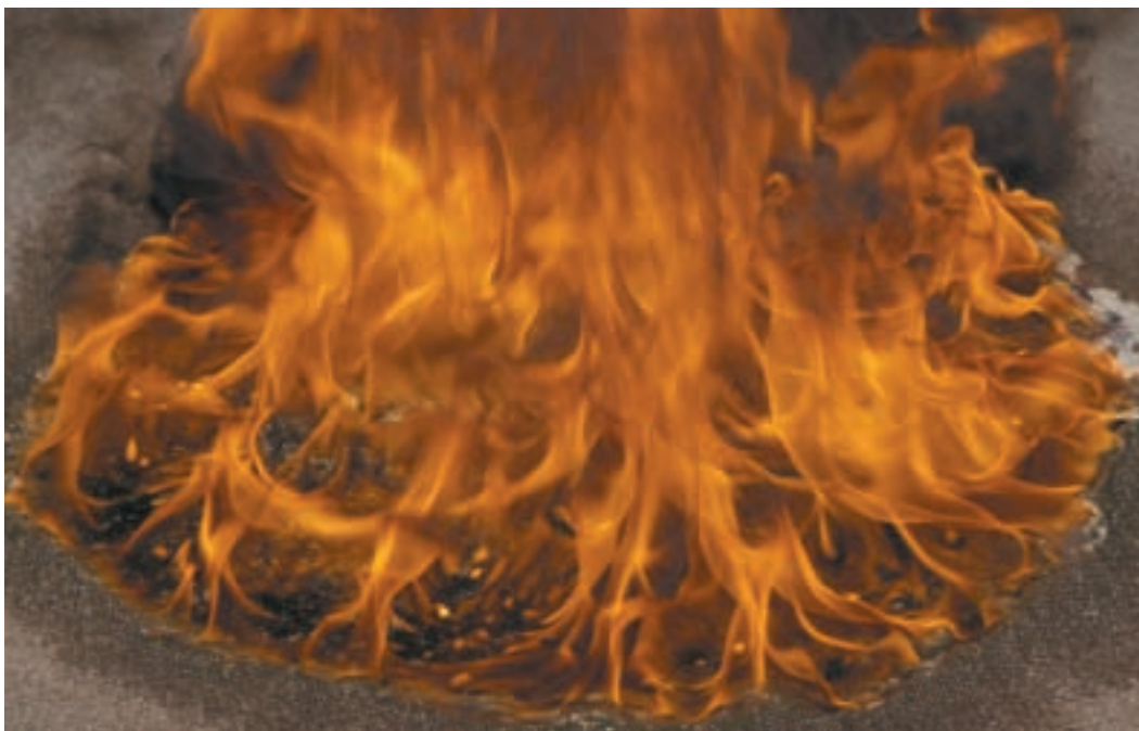
Figure 19. Closeup view of 250 mL gasoline fire on carpet 1
