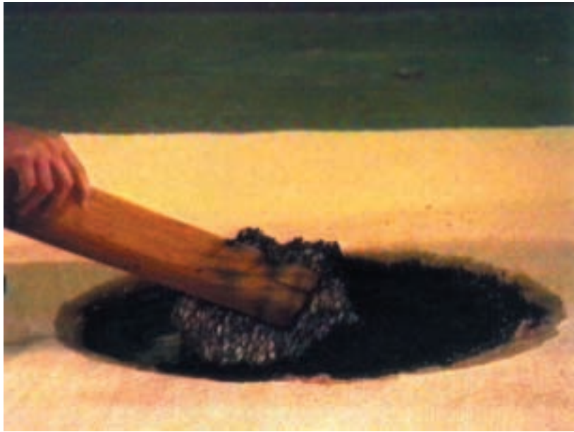
Figure 25. Carpet padding intact inside the doughnut pattern. 500 mL gasoline spill fire on carpet 2. Fire was extinguished at approximately 234 s with CO 2 .
