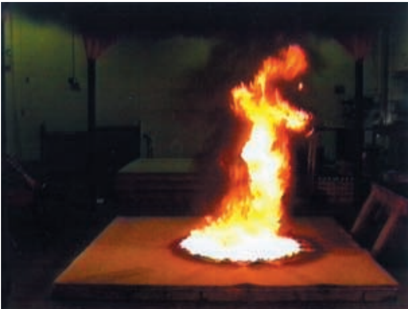
Figure 16. 1,000 mL gasoline spill fire on carpet 1 at approximately 100 s
