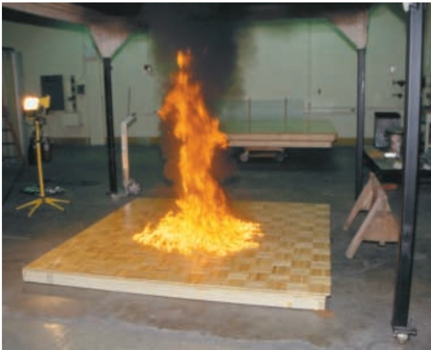
Figure 4. Gasoline spill fire under the furniture calorimetry hood in the large Fire Research Facility at NIST
