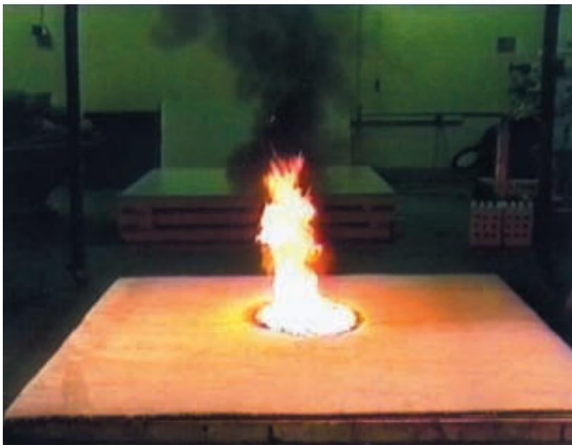
Figure 18. 1,000 mL gasoline spill fire on carpet 2 at approximately 100 s
