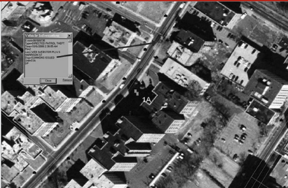
Figure 1. An aerial display in TAC-AVL, which has a zooming feature that shows the location of a patrol car and what type of call it is responding to.
