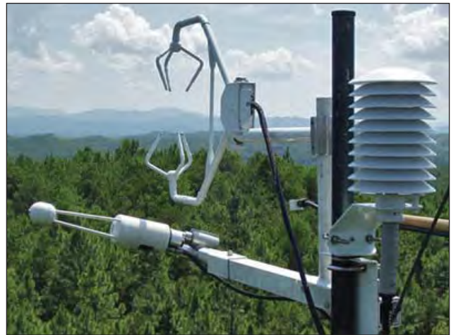
Eddy covariance tower manufactured by LICOR. Lawrence Berkeley National Laboratory leads this aspect of MVA work for the Midwest Geological Sequestration Consortium
