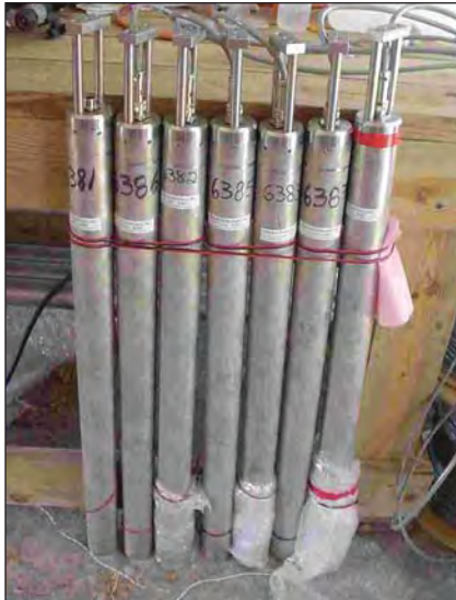
Pinnacle tiltmeter array. These devices are placed over CCS formations to monitor subsurface fluid movement and caprock integrity
