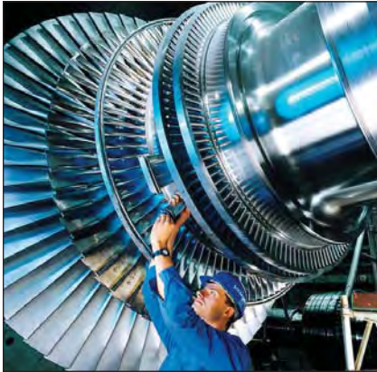
Inspection of a steam turbine rotor assembly
