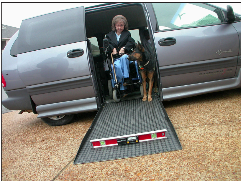
The slope of this parking space is too steep for people who use wheelchairs.
