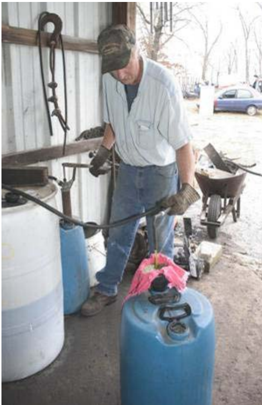
Here, antifreeze is being filtered through a homemade filtering device, to remove particulate matter before reusing it in vehicles.
