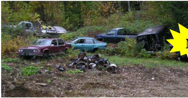
Vehicles stored in brushy areas cannot be easily inspected for leaks.
