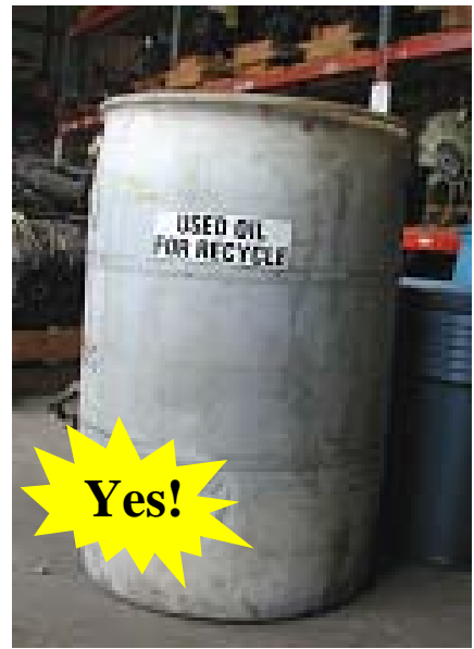
Label all used oil containers to show the contents.
