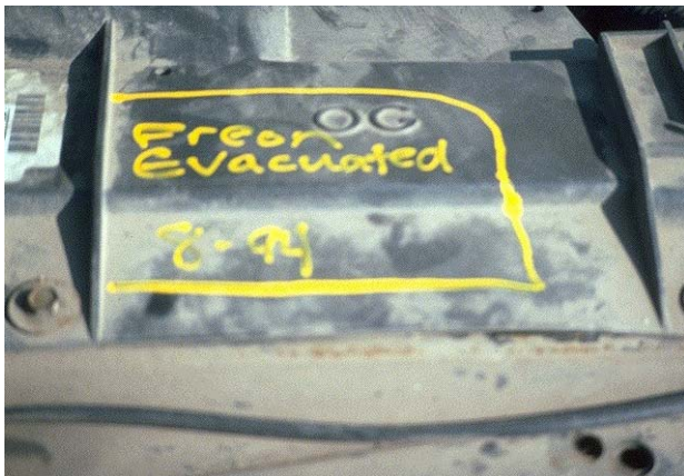
Vehicles should be marked to indicate the refrigerants have been removed.
