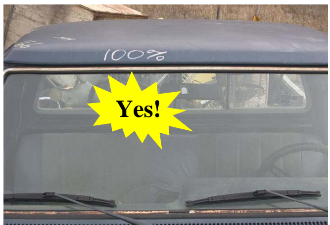
It's a good idea to clearly mark vehicles to show they have been fully drained.
