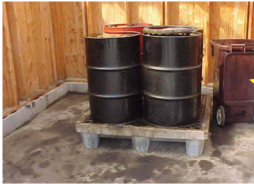
Keep tanks, drums and other fluid containers inside an enclosed structure on a leak-proof surface.
