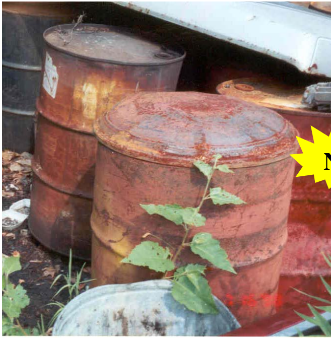
Rusted, bulging, and dented containers are not safe for storing fluids.
