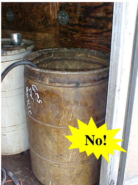
Storing gasoline in open containers is a fire and explosion hazard, in addition to being at risk for spills.
