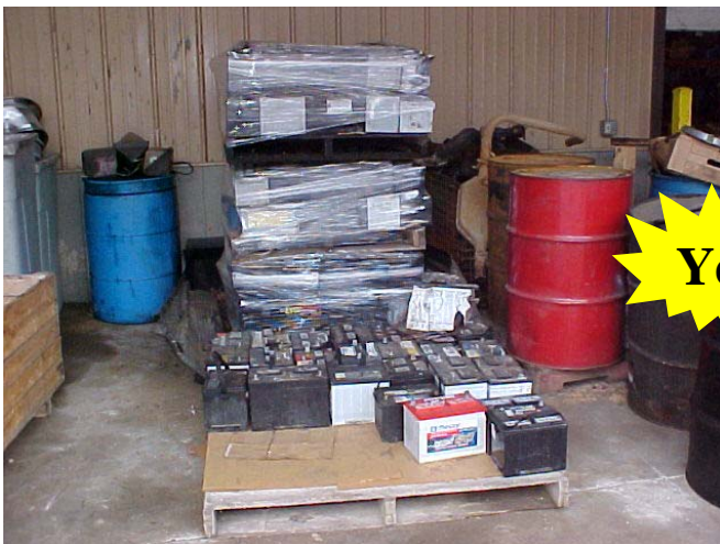
These batteries are stored correctly on a pallet inside a storage shed with a concrete floor. Cardboard is used to separate each layer. When the pallet is full, it is shrink-wrapped for shipping to a recycler.
