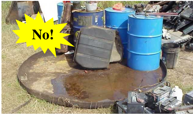
This tank bottom is not a good secondary containment device because it will not hold 110 percent of the volume of the largest container stored inside and will quickly fill with rain and melted snow.
