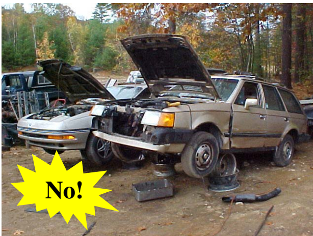
Never drain fluids over bare ground.
