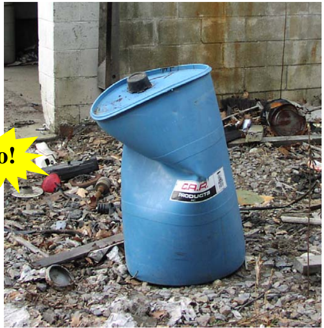
Rusted, bulging, and dented containers are not safe for storing fluids.
