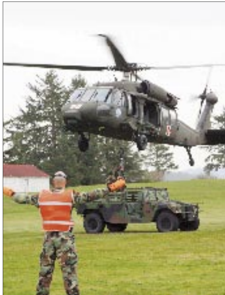
An Air Assault student marshals an Oregon Army National Guard UH-60 "Blackhawk" into position to sling-load a vehicle.
