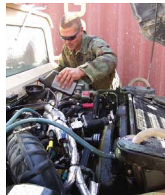
Tech. Sgt. Brian Lackman, innovative NCOIC of FOB Apache's motor pool, adds power-steering fluid to an up-armored humvee.
