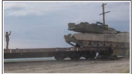
The Loadmaster for the 116 Brigade Combat Team backs an M1A1 Abrams Tank onto a railcar in preparation for movement to Ft. Bliss, Texas to train for deployment to OIF III.
