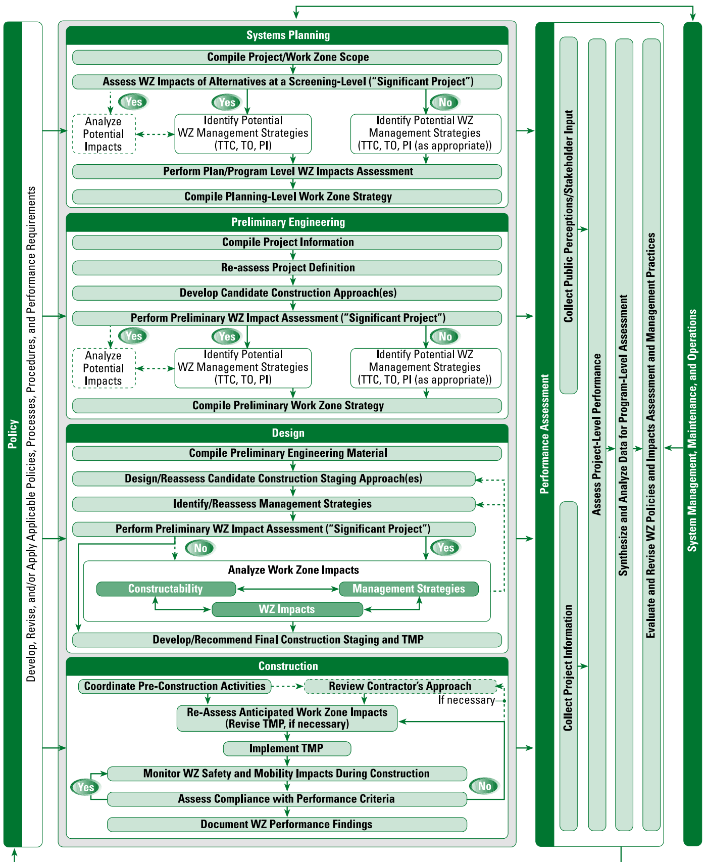
Figure 2.2 Overall Work Zone Impacts Assessment Flow Diagram
