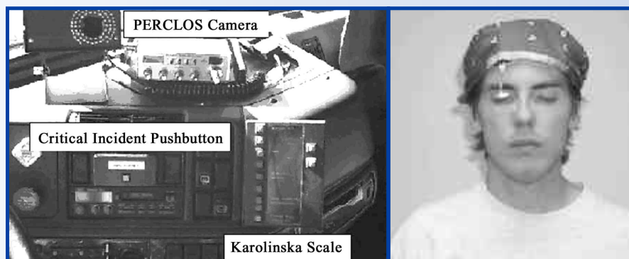
Figure 2: Instrumentation Visible to the Driver from the Driver's Seat and Nightcap Sleep Monitoring System
