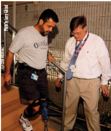
Henry Diaz, an Army veteran who lost his leg in a civilian auto accident, demonstrates the stair-handling ability of the microprocessor-controlled Rheo Knee, as Dr. Robert Gailey looks on.
