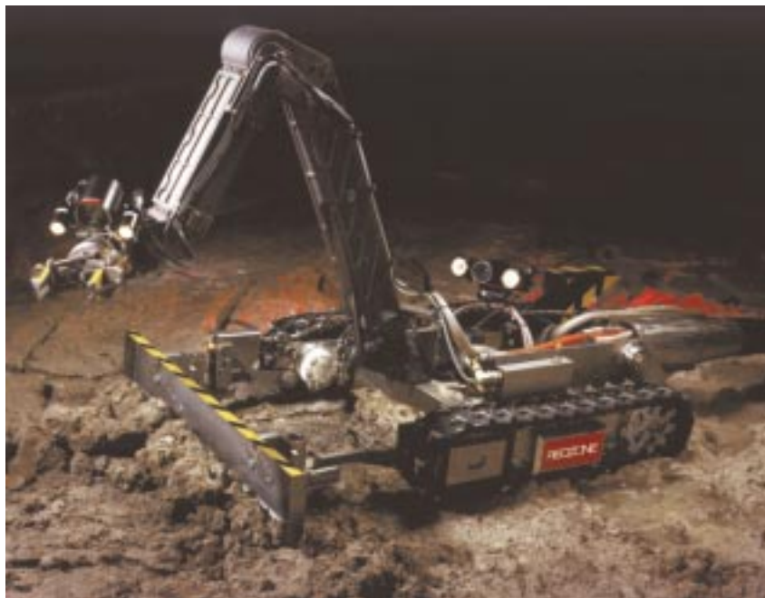
Houdini vehicle working by remote operation in a tank.
