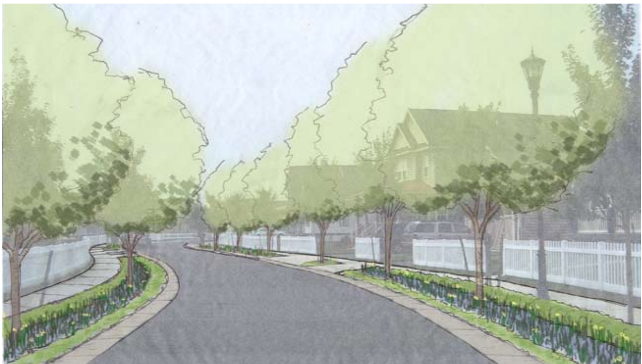
Figure 5-15: RETROFIT OPPORTUNITY: Same residential street using vegetated swales in the street's planting strips.
