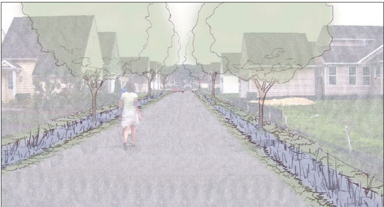
Figure 80. Retrofit potential: Side swales in a residential alley.
