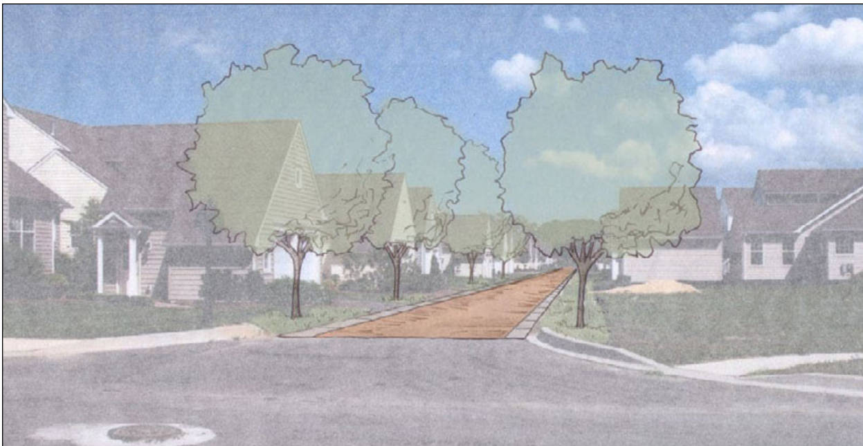
Figure 55. Retrofit potential: Complete application of pervious paving in a residential alley.
