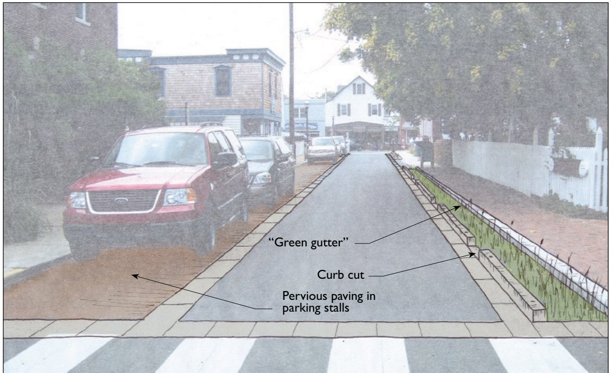
Figure 106. Retrofit potential: A “green gutter” and permeable paving in the parking zone.
