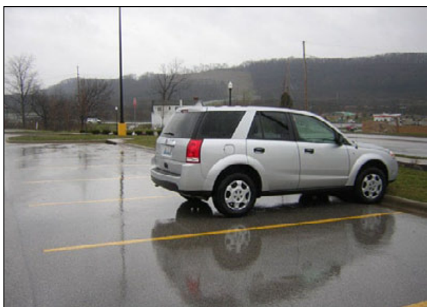
Figure 91. These oversized parking stalls could be made a few feet shorter to make room for swales.
