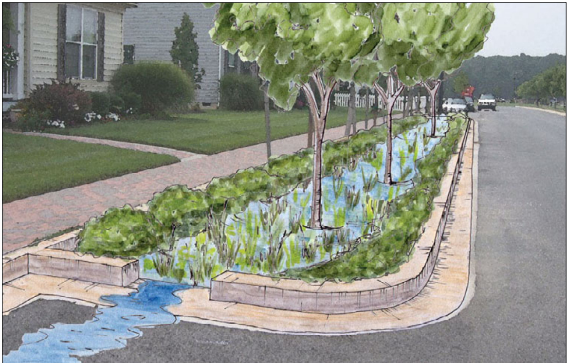
Figure 127. Retrofit potential: Planters or swales in these curb extensions could significantly improve stormwater quality and quantity.
