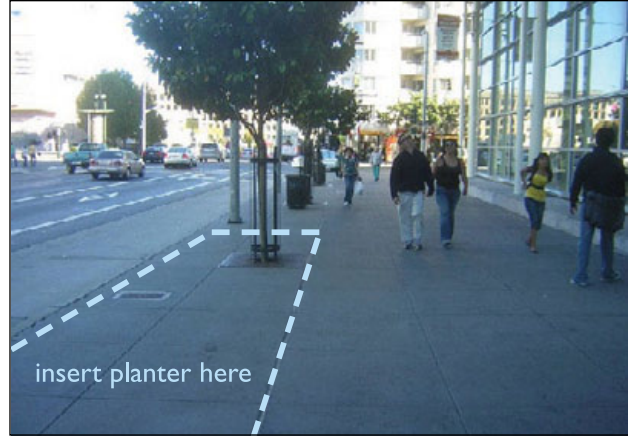
Figure 102. Planters can be retrofitted on urban streets with overly wide sidewalk zones. Dashed lines show where a planter could be added.
