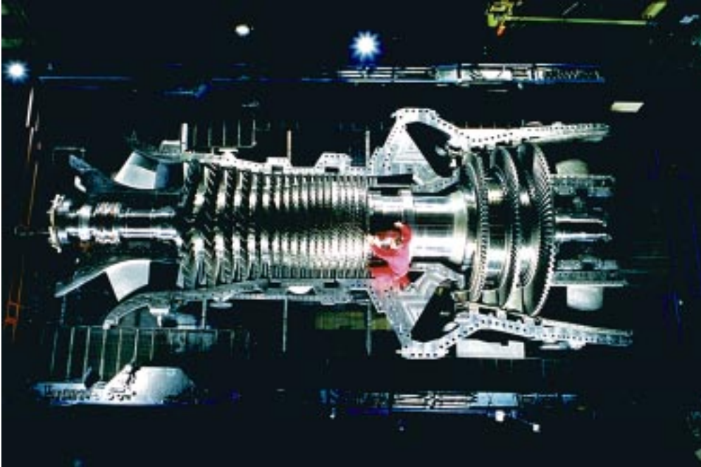
Gas turbine, model MS 7001F, during manufacture
