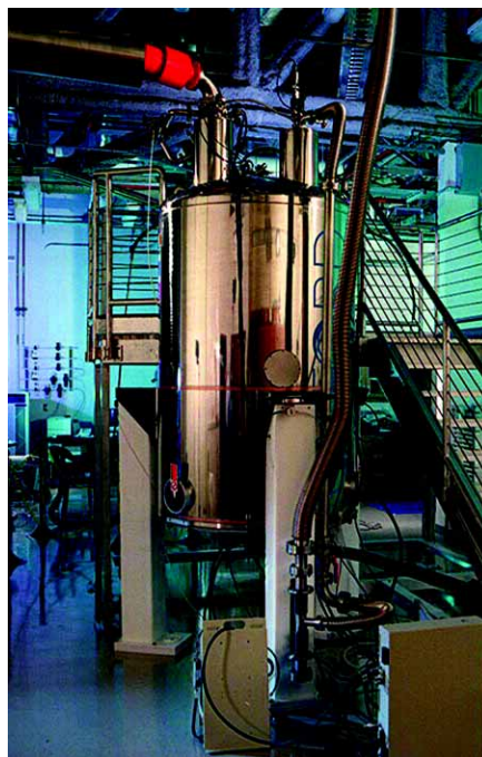
Environmental Molecular Sciences Laboratory's 800-mhz NMR spectrometer at Pacific Northwest National Laboratory
