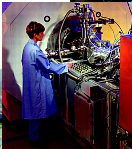
Mass spectrometer in the Environmental Molecular Sciences Laboratory at Pacific Northwest National Laboratory
