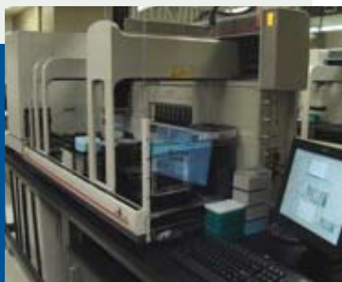
BESC Biomass Characterization Pipeline. Processing more than 1,000 biomass samples per week, the BESC pipeline's high-throughput assays for enzyme deconstruction are used to assess recalcitrant features of biomass samples and screen for more effective enzymes.
