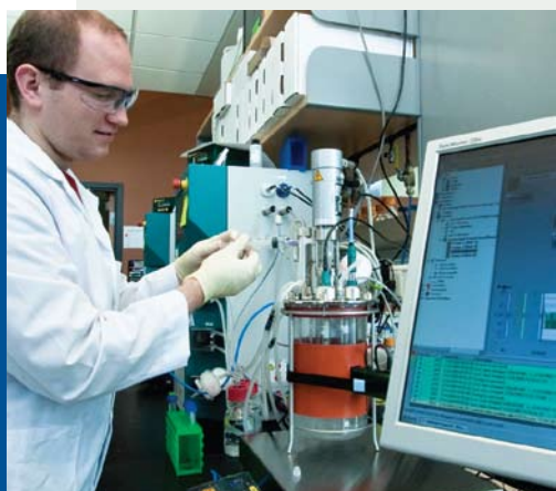
GLBRC Microbial Screening. Wesley D. Marner, II, works with highly instrumented bioreactors to study experimental fermentation and microbial production of biofuels at cellular and reactor scales. [Photo by Wolfgang Hoffmann, University of Wisconsin–Madison]
