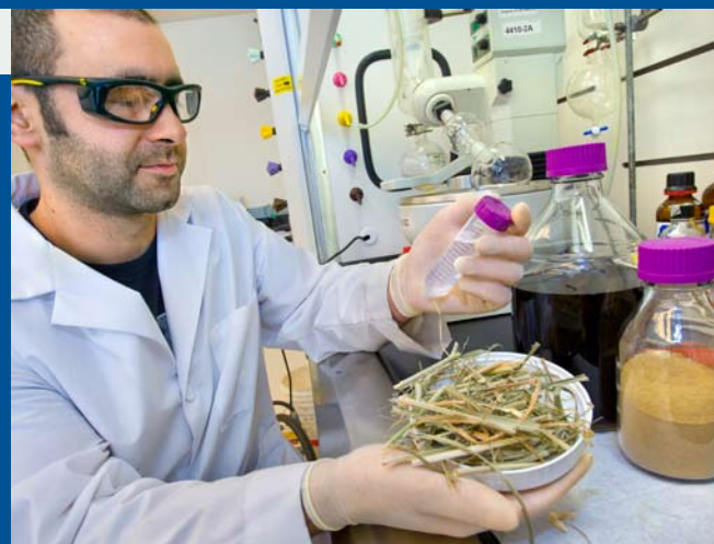
JBEI Ionic Liquid Pretreatment Research. Brad Holmes studies ionic liquids—the focus of a new pretreatment approach that has a unique capacity for dissolving lignocellulosic biomass and helping to hydrolyze the resulting liquor into sugars for biofuel production.
