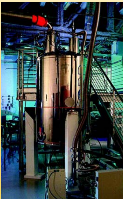
Environmental Molecular Sciences Laboratory's 800-MHz nuclear magnetic resonance spectrometer at Pacific Northwest National Laboratory
