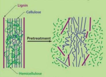
Cellulose exists within a matrix of other polymers, primarily hemicellulose and lignin. Pretreatment of biomass with heat, enzymes, or acids removes these polymers from the cellulose core before hydrolysis.
