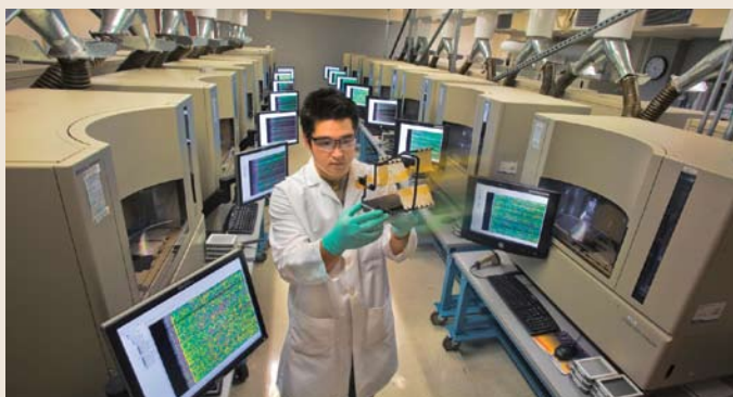
High-Throughput DNA Sequencing. Automated machines at the DOE JGI Production Genomics Facility sequence millions of DNA base pairs per day.
